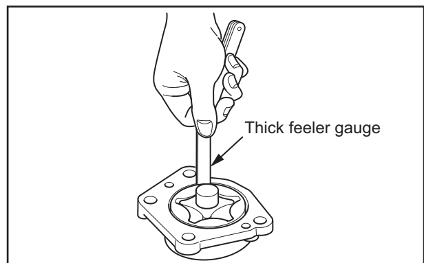
Measuring clearance between outer rotor and pump case
