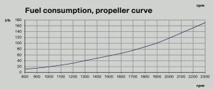
Test conditions. Air temperature +25 °C. Barometric pressure 100 kPa (750 mmHg). Humidity 30%. Diesel fuel acc.to ECE R 24 Annex 6. Density of fuel 0,840 kg/dm³. Viscosity of fuel 3.0 cSt at 40 °C. Energy value 42,700 kJ/kg. Power test code ISO 3046. Power and fuel values +/-3%.
