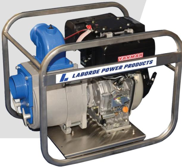
Laborde Products offers a series of cast iron solids handling pumps in 2" and 3" configurations for heavy duty applications. All pumps are mounted on vibration isolators and enclosed in an aluminum roll cage. Trash pumps feature heavy duty cast iron impellers. Pumps are powered by the Yanmar L70W air cooled diesel engine. Available with optional stainless steel roll cage.
